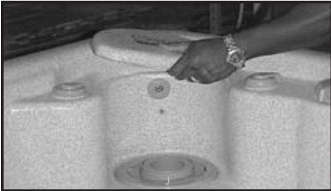
1. Activate the standby mode or turn off electrical power. Remove filter cover and set aside.
